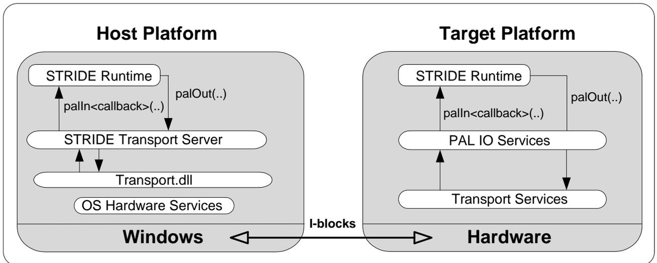
**Figure 2. Transport Block Diagram****2.2. Host Services**
